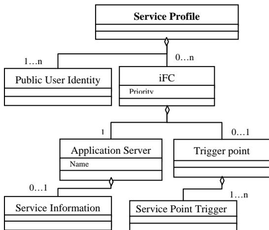
Figure 4: IMS user Service Profile defined by 3GPP
