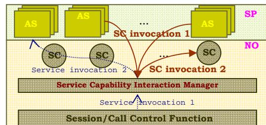
Figure 2: Proposed Service Invocation Mechanism
