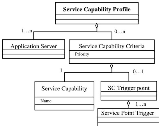
Figure 5: Proposed Service Capability Profile of AS
