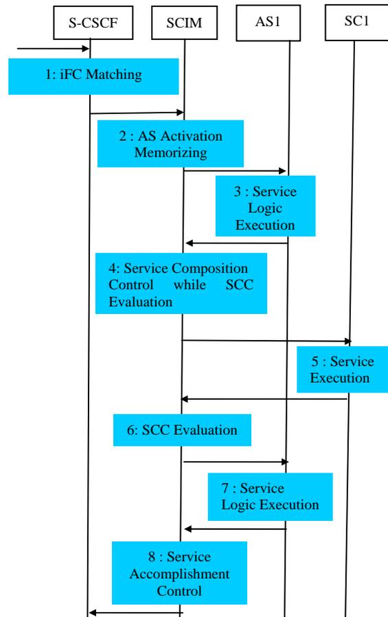
Figure 6: Controlling the Service Capability Composition
