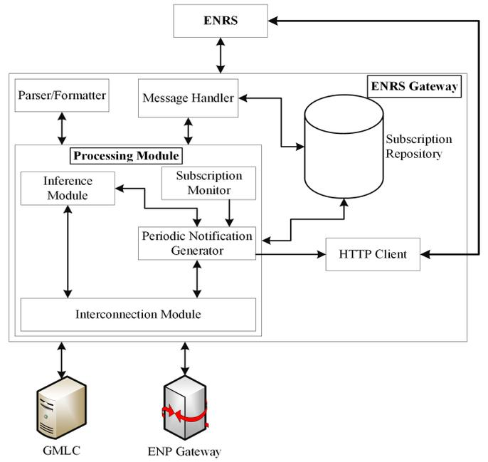
Fig. 2. ENRS Gateway architecture
